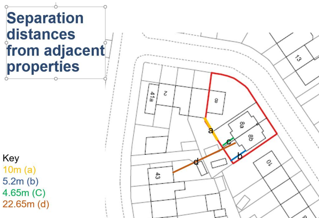
Fig 2: Separation distances from adjacent properties
